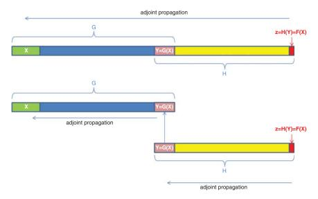
It should be clear that an overall back-propagation through the entire tape of F is equivalent, and produces the same results, as two successive back-propagations, first through the tape of H, and then through the tape of G. Note that the order is reversed from evaluation, where G is evaluated first and H is evaluated last.
