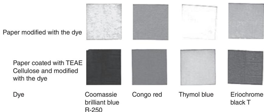
**Figure 1.17** Images of printing paper coated with amino cellulose and subsequent coloring. (See insert for color representation of this figure.)
